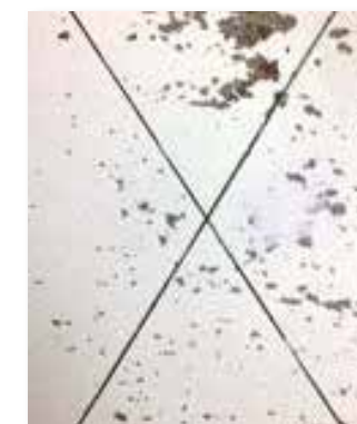
Paint applied to aluminum with pre-treatment A shows minimal adhesion failures
